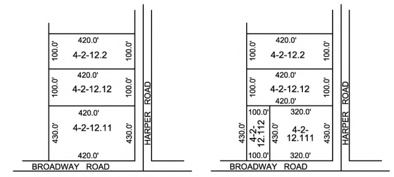
3. WHEN A PARCEL IS RESUBDIVIDED SUCH AS 4-2-12.1, THE PARCEL SOLD OFF BECOMES 4-2-2.12 AND THE RETAINED PORTION BECOMES 4-2-12.11.
