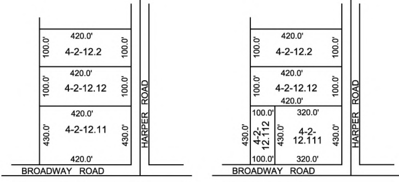
3. WHEN A PARCEL IS RESUBDIVISIONED SUCH AS 4-2-12.1, THE PARCEL SOLD OFF BECOMES 4-2-2.12 AND THE RETAINED PORTION BECOMES 4-2-12.11.
